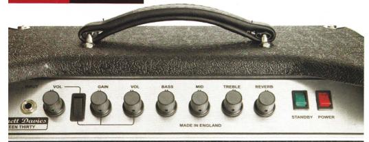
Clean, simple front panel, and well kicked back to protect the knobs
